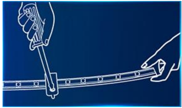
2. Tighten the mounting clip with M3*6 screws
